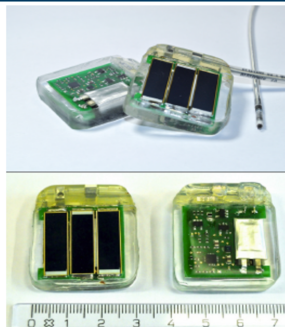
Figure 2 The sunlight-driven pacemaker prototype 2 (2 devices are shown). Top , A conventional bipolar active pacemaker lead (Safio S60, Biotronik) is attached via an IS-1 header. Bottom , The back side of the device reveals a small lithium-polymer accumulator (visible as silver part of the device on the right). The energy source for the device, a solar module, can be seen in the frontal view (device on the left). The dimensions of the device are 30 × 35 × 6 mm.
